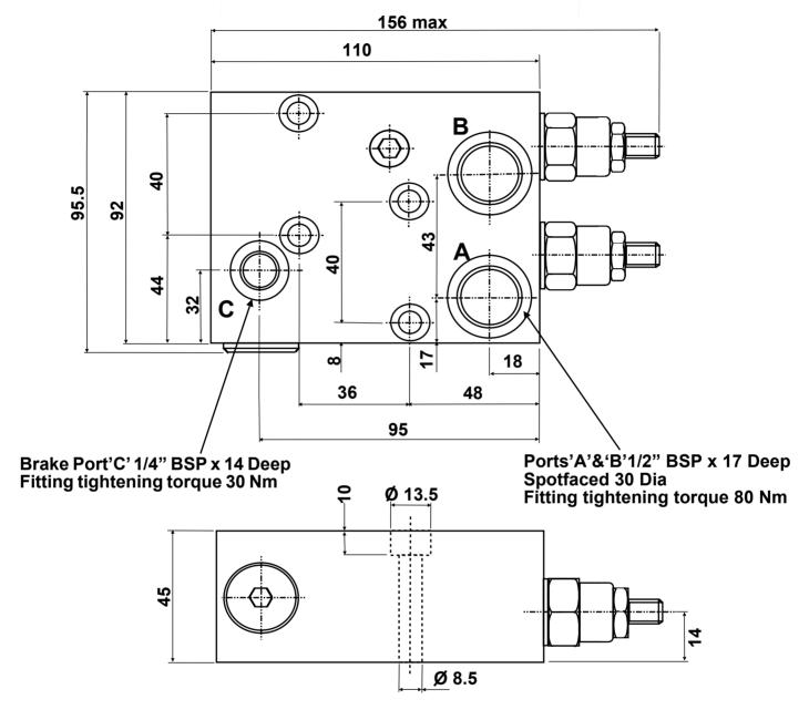
Maximum pressure 280 bar 4060 psi Pressure range 60-280 bar 870-4060 psi Maximum rated flow 60 lpm Pilot ratio 4.25:1 Valve supplied complete with mounting screws & 'o' rings. Valves are not pre-set Should a set pressure be required please state at time of order.
